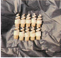
AFTER CLEANING SPRAY NOZZLE
