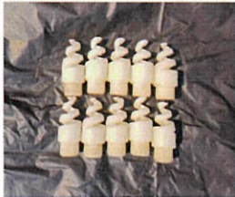
AFTER CLEANING SPRAY NOZZLE
